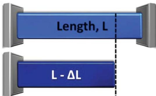
Figure 2: Contraction of a glass bar due to uniform, slow cooling.
