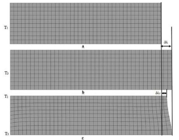
Figure 5: FEA response to heating the lower surface of a cold glass bar.
