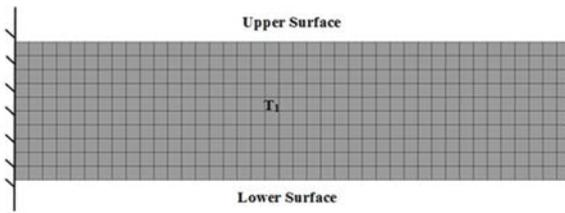
Figure 3: Finite element model of a glass bar subjected to thermal shock.
