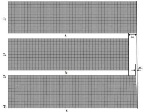
Figure 4: FEA response of cooling the upper surface of a hot glass bar.
