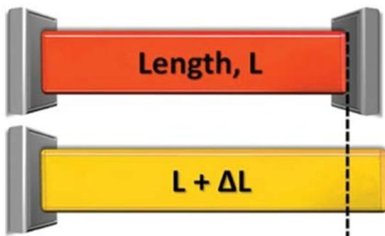
Figure 1: Expansion of a glass bar due to uniform, slow heating.
