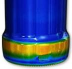
container. Otherwise, simply moving glass from one area to the heel contact point may result in thin glass at another critical region that could then become problematic. Thus, the most effective solution will be to re-design the container to reduce the magnitude of the vertical load stress index at the heel contact point.
