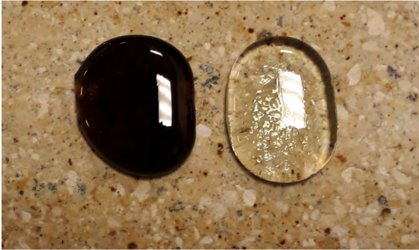
Figure 4.27: The sample 60\text{KPO}_3\text{-}20\text{slag-}20\text{Al}_2\text{O}_3 , melted at temperatures varying from 1250^\circ\text{C} to 1500^\circ\text{C} .
