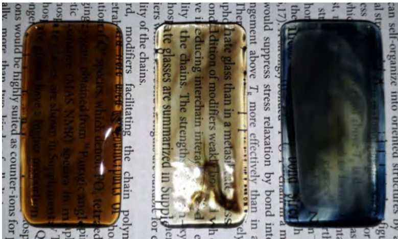
Figure 4.10: Samples consisting of 15% slag, without the addition of B_2O_3 , with the addition of 10% B_2O_3 and 20% B_2O_3 , respectively.
