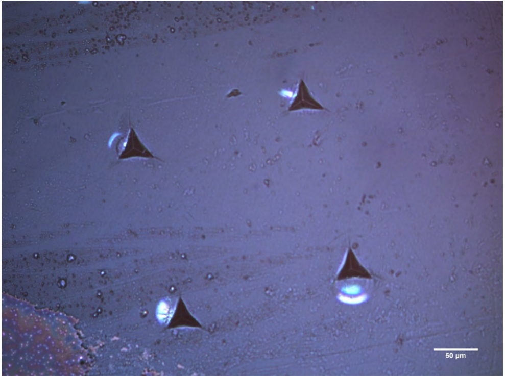
Figure E.21: Sample 75KPO 3 -12.5slag-12.5Al 2 O 3 under 2N analysed by reflected light.
