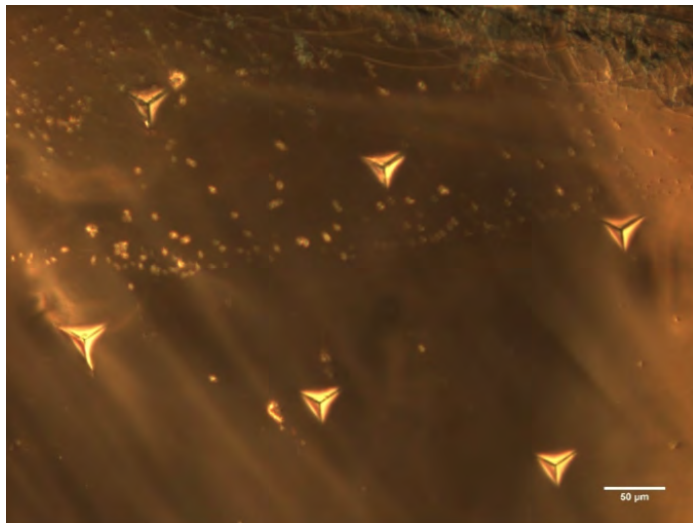
Figure E.8: Sample 40\text{KPO}_3\text{-}20\text{B}_2\text{O}_3\text{-}25\text{FA-}15\text{Al}_2\text{O}_3 under 2.N.
