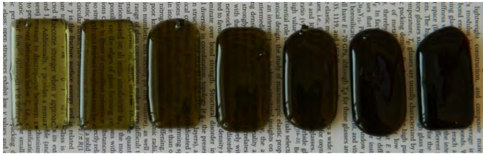
Figure 4.11: The samples containing fly ash (FA) - From the left to the right: 75KPO 3 -12.5FA-12.5Al 2 O 3 , 70KPO 3 -15FA-15Al 2 O 3 , 65KPO 3 -20FA-15Al 2 O 3 , 60KPO 3 -20FA-20Al 2 O 3 , 60KPO 3 -25FA-5Al 2 O 3 , 60KPO 3 -30FA-10Al 2 O 3 , 55KPO 3 -35FA-10Al 2 O 3 .
