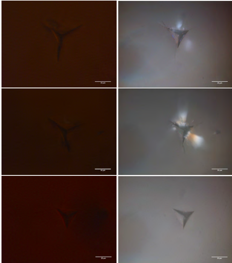
Figure E.32: Three indents of the sample 60\text{KPO}_3\text{-}20\text{slag-}20\text{Al}_2\text{O}_3 under 2N, analysed by transmitted (left) and reflected light (right).
