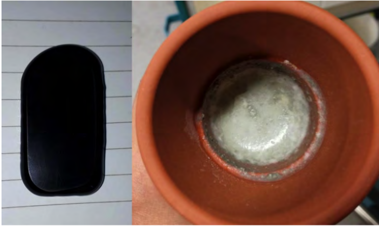
Figure 4.20: The sample 60\text{KPO}_3\text{-}20\text{slag-}20\text{Al}_2\text{O}_3 produced, respectively, via the melt-quenching and the kiln-casting method.
