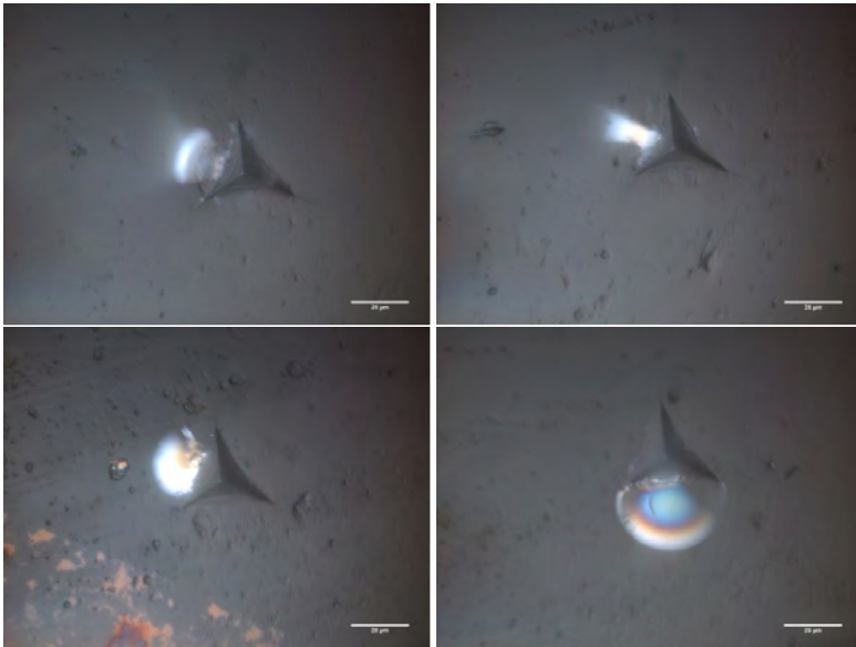
Figure E.22: Four indents of the sample 75\text{KPO}_3 - 12.5\text{slag} - 12.5\text{Al}_2\text{O}_3 under 2.N analysed by reflected light.
