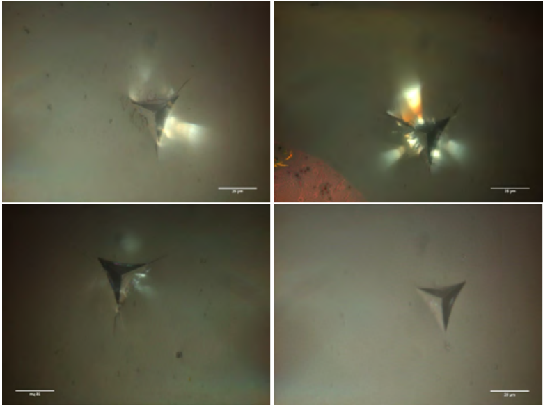
Figure E.14: Four indents of the sample 60\text{KPO}_3\text{-}20\text{FA-}20\text{Al}_2\text{O}_3 under 2.N, analysed by reflected light.
