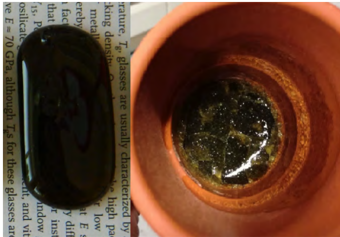
Figure 4.22: The sample 60\text{KPO}_3\text{-}30\text{FA-}10\text{Al}_2\text{O}_3 produced, respectively, via the melt-quenching and the kiln-casting method.
