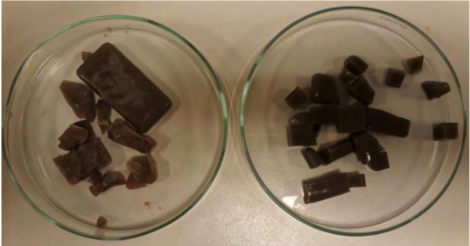
Figure 3.7: Non-transparent samples containing 80KPO 3 .20Slag and 70KPO 3 .30Slag, respectively.
