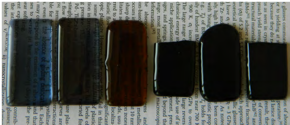
Figure 4.8: The samples containing slag. From the left to the right: 77.5\text{KPO}_3\text{-}10\text{Slag-}12.5\text{Al}_2\text{O}_3 , 75\text{KPO}_3\text{-}12.5\text{Slag-}12.5\text{Al}_2\text{O}_3 , 70\text{KPO}_3\text{-}15\text{Slag-}15\text{Al}_2\text{O}_3 , 65\text{KPO}_3\text{-}17.5\text{Slag-}17.5\text{Al}_2\text{O}_3 , 65\text{KPO}_3\text{-}20\text{Slag-}15\text{Al}_2\text{O}_3 , 60\text{KPO}_3\text{-}20\text{Slag-}20\text{Al}_2\text{O}_3 .
