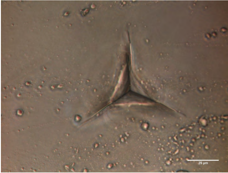
Figure 6.12: Indent of the sample 75\text{KPO}_3\text{-}12.5\text{slag-}12.5\text{Al}_2\text{O}_3 .
