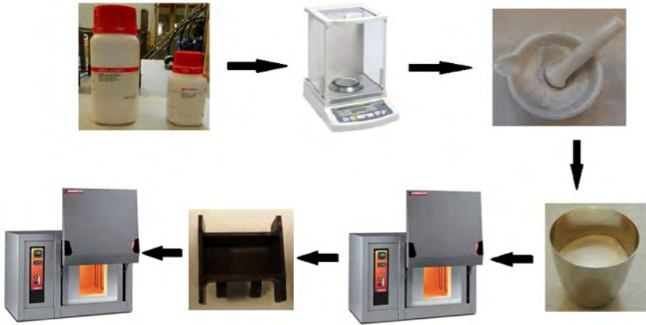
Figure 3.5: Scheme of the glass samples production: preparation of the batch, melting, quenching and annealing.
