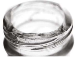
Figure 5: Representative fracture pattern.
