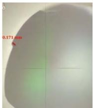
Figure 10: Overmatch measuring 0.17mm.
