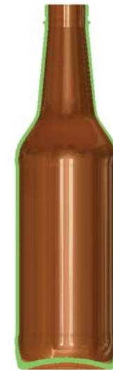
Figure 1: 3D Solidworks model for a 330ml bottle. The green coloured region represents the thickness distribution.
