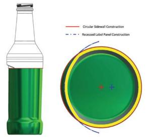
Figure 3: Construction of a recessed label panel.
