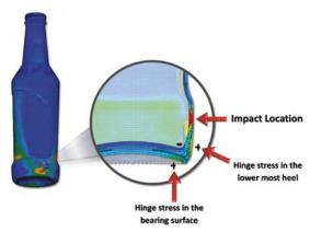
Figure 4: Hinge stresses with complex curvature.
