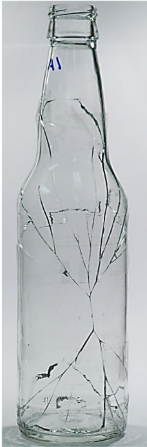
A1 Internal Pressure Sidewall Origin
