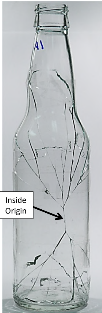
A1 Internal Pressure Inside Surface Origin
