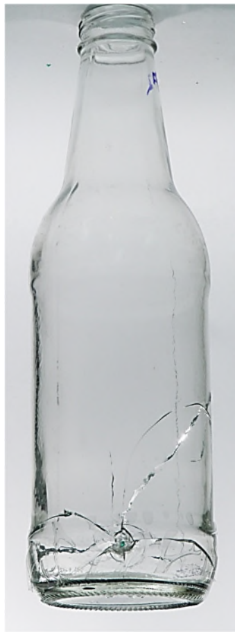
F2 Impact Sidewall Origin
