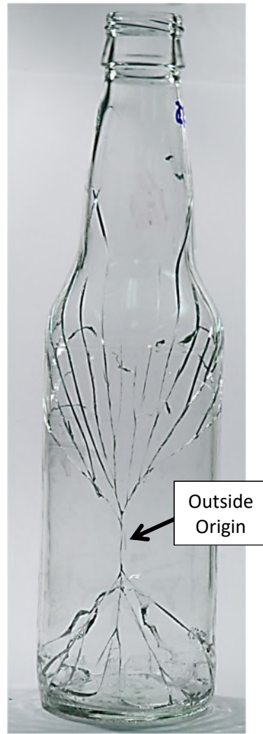
B5 Internal Pressure Outside Surface Origin
