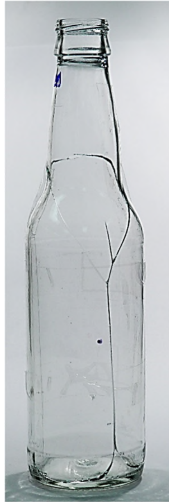
B1 Long Initial Split Low Load Level
