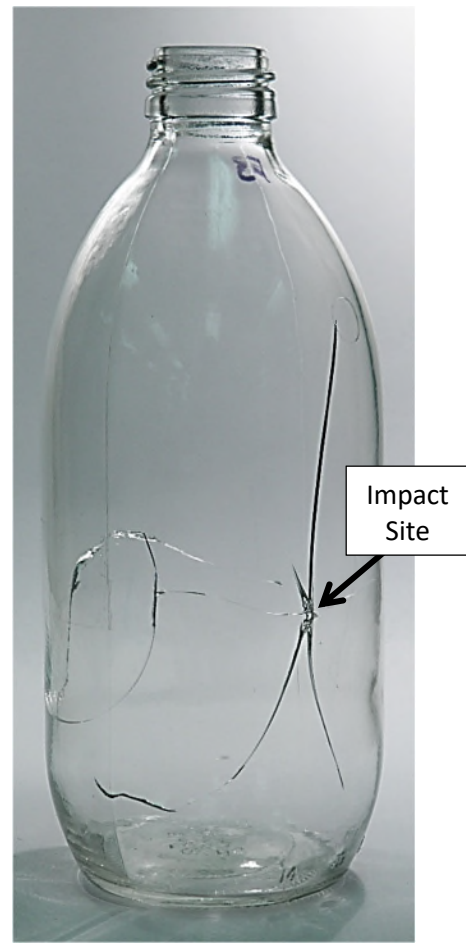
FIGURE 7 Similar Fracture Patterns with Different Breakage Modes F4 – Flexure with Inside Origin F3 – Sidewall Hinge with Outside Origin
