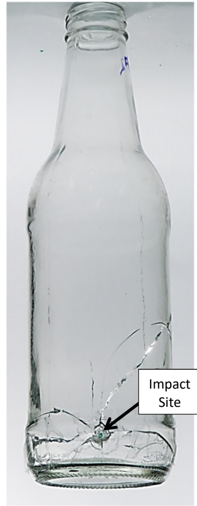
F2 – Flexure at Heel Contact
