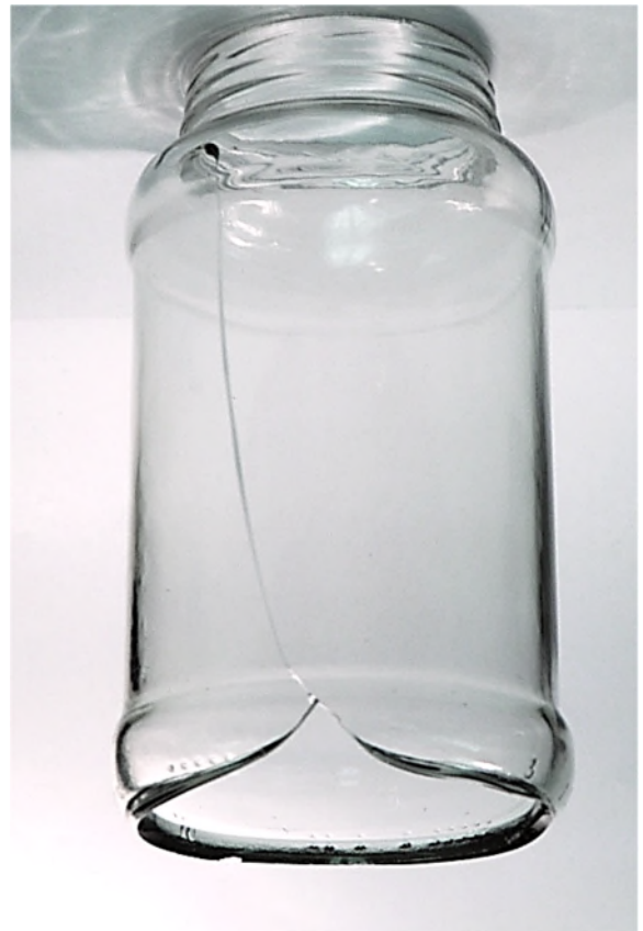
H2 Thermal Sidewall Origin
