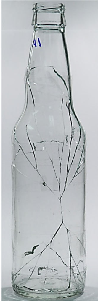
A1 Short Initial Split High Load Level
