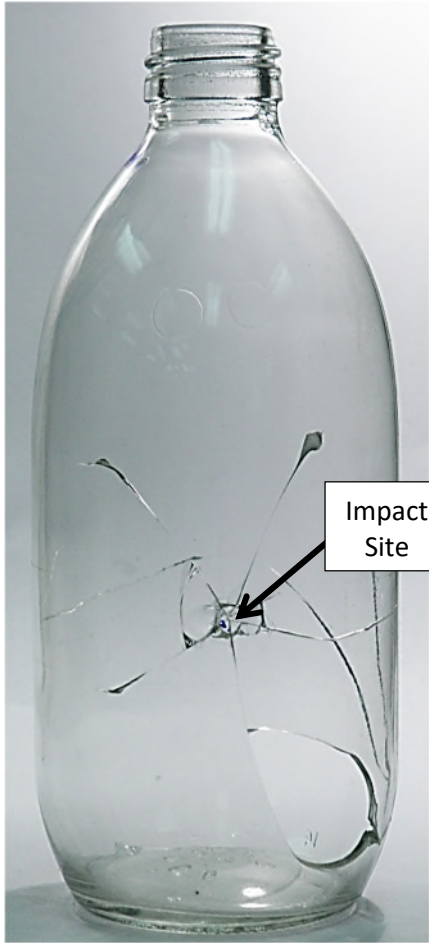
FIGURE 7 Similar Fracture Patterns with Different Breakage Modes F4 – Flexure with Inside Origin F3 – Sidewall Hinge with Outside Origin
