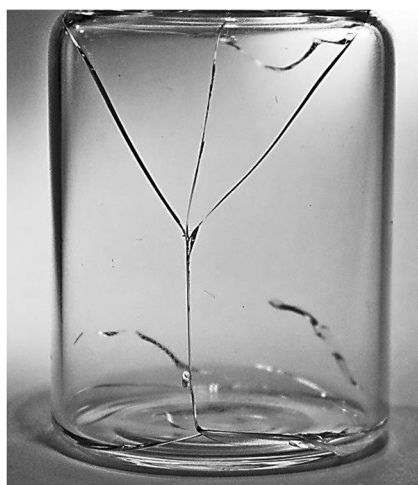
a) Failure at relatively high pressure
