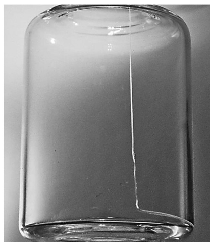
b) Failure at relatively low pressure
