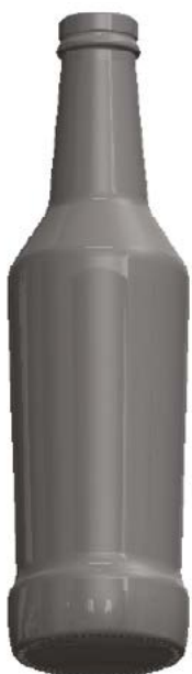
Figure 1: FEA model of a generic 330ml bottle.
