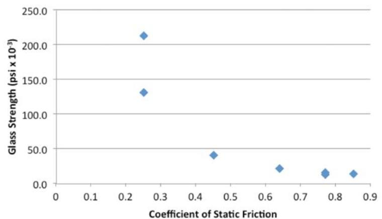
Figure 2: Resultant glass strength as a function of friction.
