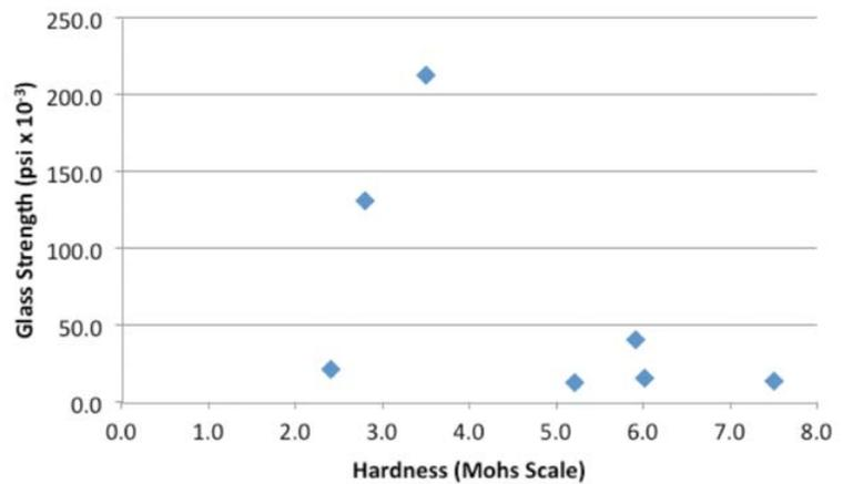
Figure 1: Resultant glass strength as a function of metal hardness.
