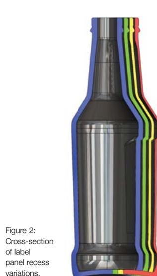
Figure 2: Cross-section of label panel recess variations.
