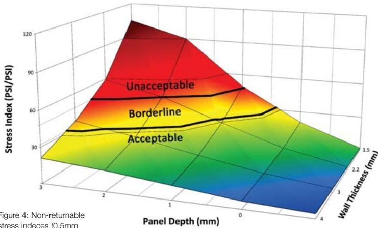
Figure 4: Non-returnable stress indices (0.5mm transition radius).
