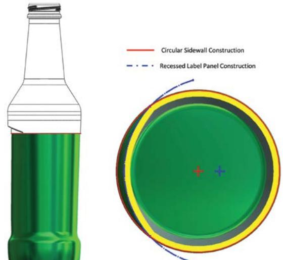
Figure 3: Construction of a recessed label panel.
