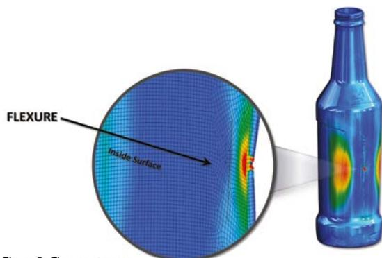
Figure 2: Flexure stresses.
