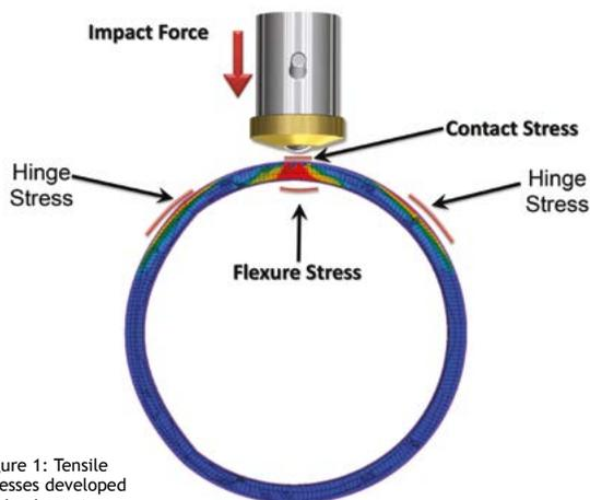
Figure 1: Tensile stresses developed during impact.
