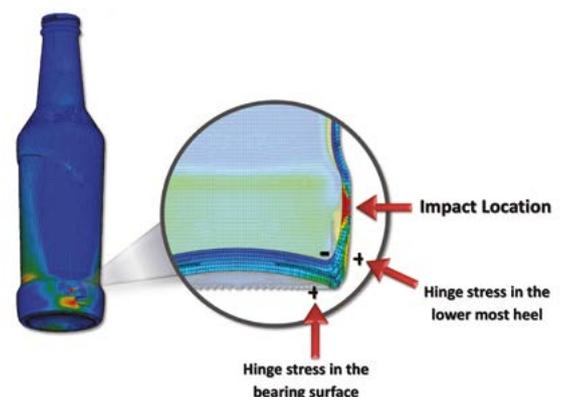
Figure 4: Hinge stresses with complex curvature.
